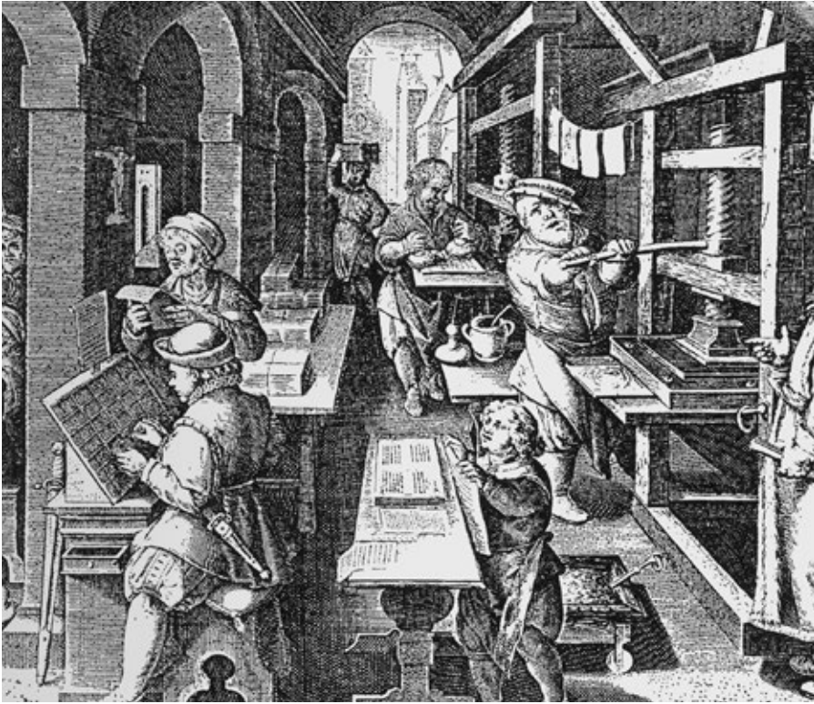
Plate 5. This late sixteenth-century printer's shop would have been equally typical of the preceding century. Note the press-man at a screw-type press, another man inking the type with two large pads (rear centre), and the correction of the type in the forme (left foreground). From a wood-block engraving by the Dutch artist Jan van der Straat ('Stradanus', 1536–1604).
